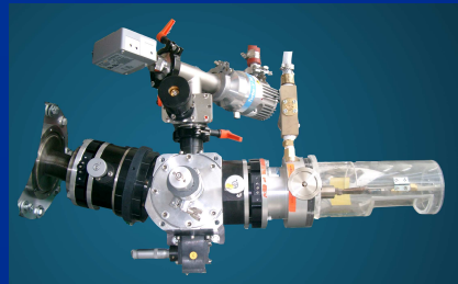
The image above shows the EUV plasma source on the right connected to the new grazing incidence monochromator in the center. On the left is the entrance to the octagonal chamber.
